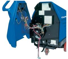
Electronic components are all easily accessible via a hinged access door. All components are simple to service.
