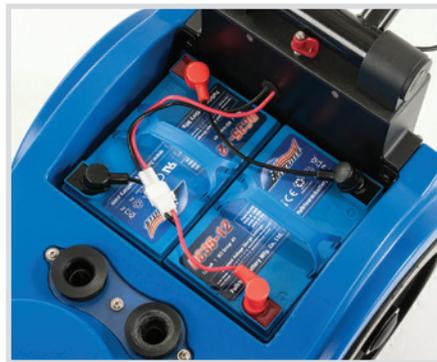
Maintenance-free AGM batteries and onboard charger.
