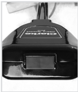
Safety lock-out switch.
