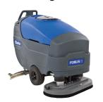
The Focus® II Large walk-behind autoscrubber® has the right combination of capacity, cleaning path, runtime, and rugged durability desired by contractors, rental companies and industrial facilities. With 30 gallons (114 L) of solution capacity and a 34 inch (86 cm) scrub path you will be able to tackle the largest jobs quickly and efficiently.
