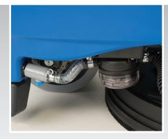
**Solution Filter**Externally mounted solution filter is easy to clean and minimizes exposure to chemicals.
