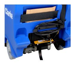
Onboard battery charging permits charging the batteries at any convenient location with a 120 V outlet. Also features storage for extra dust filtration bags.
