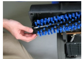
The 16 or 18 inch scrub brush can be removed and installed without the use of tools.
