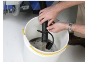
High dump drain into toilet or bucket.
