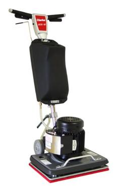
The BOS-18 is used for scrubbing and chemical-free stripping. The powerful, totally enclosed motor requires less maintenance, and provides for 3,600 1/4 inch orbits per minute. The BOS-18 is made of heavy cast components that provide durability and weight for aggressive scrubbing and stripping agitation. A 4 gallon solution tank feeds cleaning solution to the pad.
