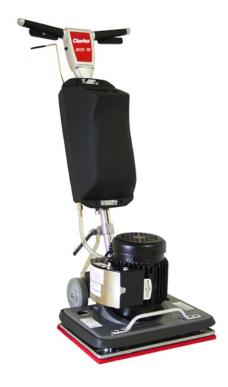
The BOS-18 is used for scrubbing and chemical-free stripping. The powerful, totally enclosed motor requires less maintenance, and provides for 3,600 1/4 inch orbits per minute. The BOS-18 is made of heavy cast components that provide durability and weight for aggressive scrubbing and stripping agitation. A 4 gallon solution tank feeds cleaning solution to the pad.
