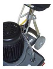
Solution is applied to the pad when released by a manual trigger on the 4 gallon solution tank.
