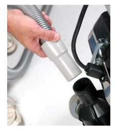
A vacuum-ready dust pipe design easily fits a 1.5 inch vacuum hose for use with a dust control vacuum system.
