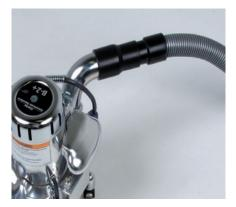
Replace the bag with the hose adaptor and the edger can be easily hooked up to a 1-1/2 inch vacuum hose.
