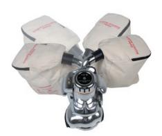
Rotating dust pipe allows the dust bag or hose connection to move freely during operation. The Super 7R pipe rotates 210° and the B-2+ pipe rotates 260°.
